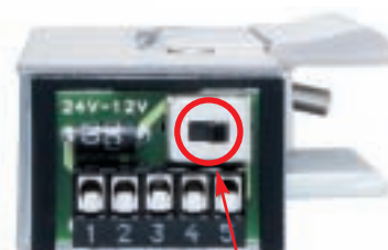
Sliding switch for voltage selection
